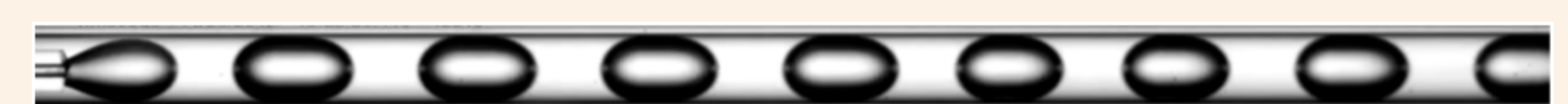
Figure – P = 20 \text{ MPa} ; T = 308 \text{ K} ; V_{\text{CO}_2} = 0.02 \text{ mL/min} ; V_{\text{H}_2\text{O}} = 0.02 \text{ mL/min} in a 530 \mu\text{m} capillary. [Region A] [1]
